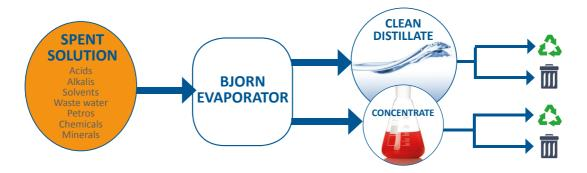
**The BJORN evaporator:** From mixed liquid to re-usable material or manageable liquid waste
